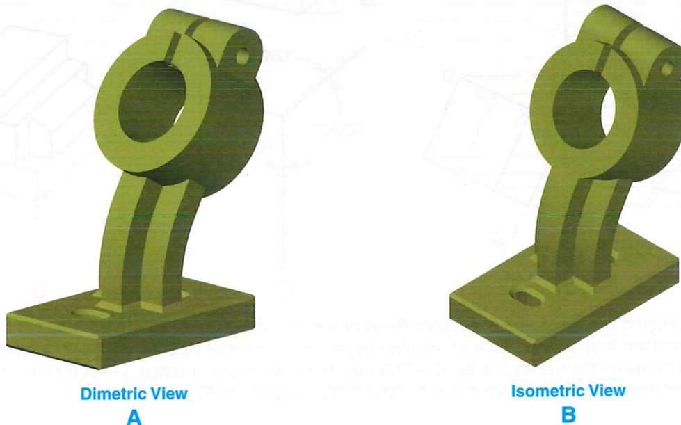
Figure 11-35. A dimetric drawing can be created in CAD by constructing a 3D model and using 3D viewing commands to set the viewing direction. Note the difference between the two views shown here. A—A dimetric drawing of a mechanical assembly. B—An isometric view of the same model shown for reference.
