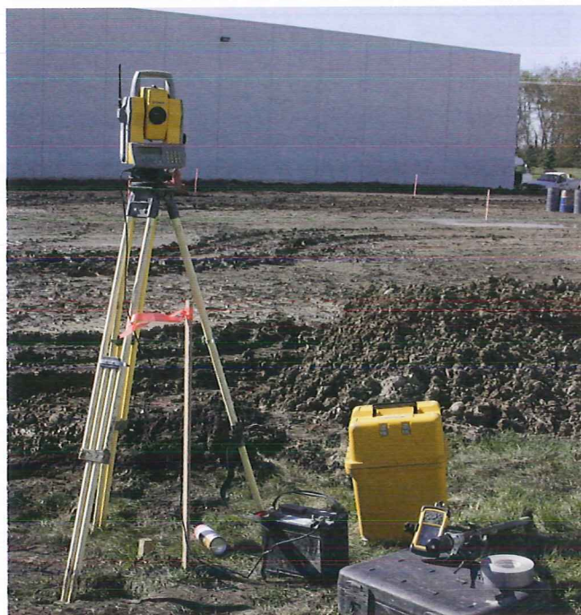
Figure 25-9. Despite the introduction of newer technology, surveying tools designed for use on the job site are still in wide use. Shown is a tripod-mounted “total station” equipped with electronic distance measurement (EDM) and leveling functions. This type of equipment is used by surveyors to take accurate measurements of land features.
