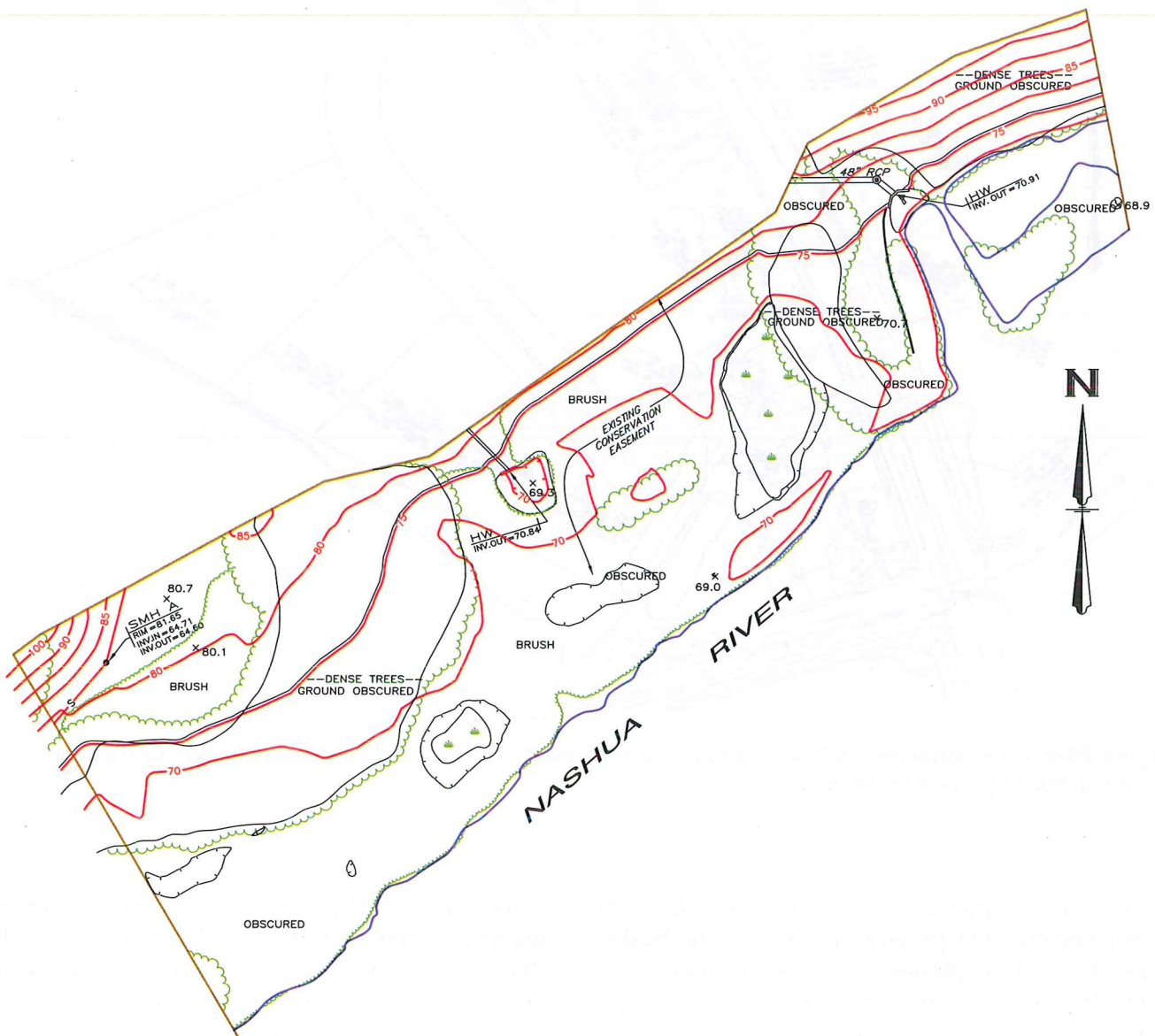
Figure 25-5. A topographic map shows contour elevations, natural features, and constructed features. Shown is a portion of a CAD-generated topographic map. (Autodesk, Inc.)
