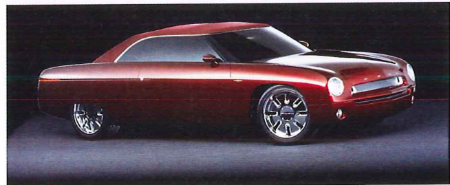
Figure 1-13. An automotive prototype is a full-size operating model of a new product idea. (Ford)
