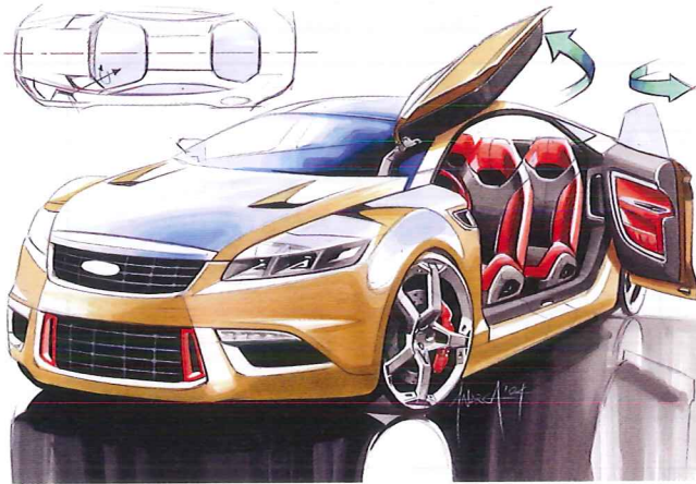
Figure 1-6. Special types of technical drawings are commonly used in advertising or promotional literature to communicate a prospective design. (Ford)
