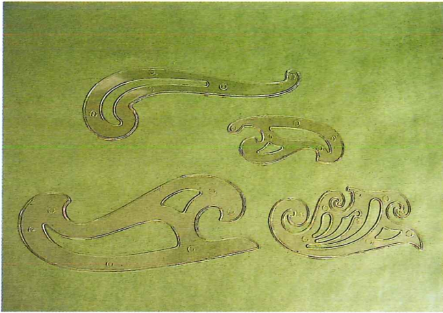
Figure 2-62. Irregular (or French) curves are available in many shapes and sizes.
