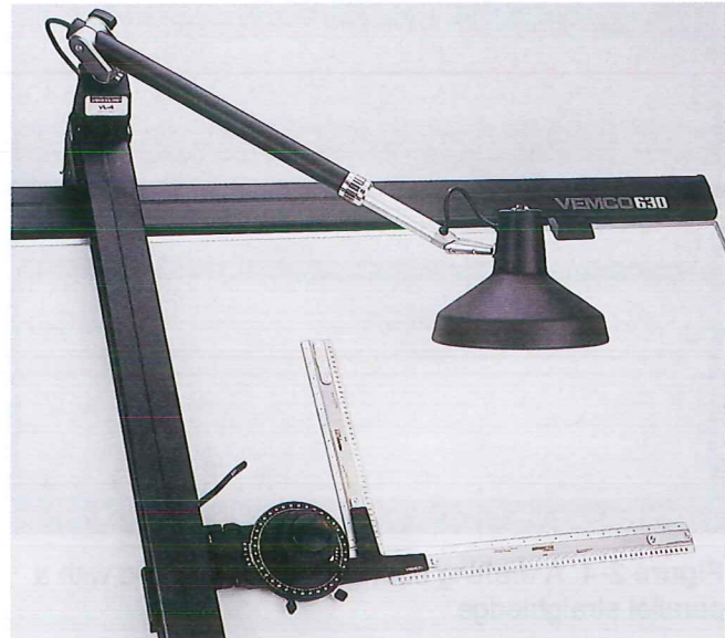
Figure 2-8. A track-type drafting machine. (Vemco Corporation)
