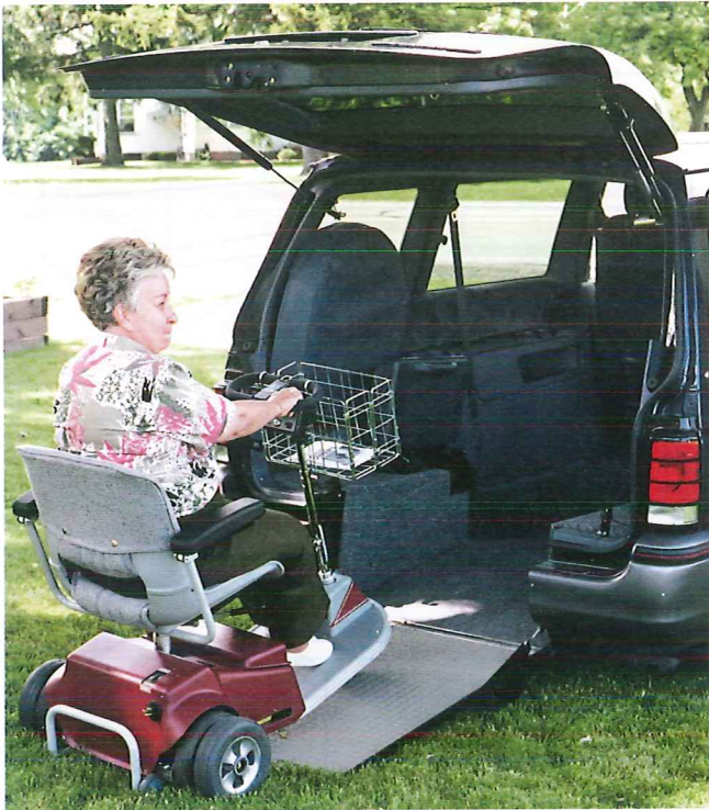
Figure 12-9. There are specific requirements that must be met when designing vehicles for handicapped individuals. The slope of an access ramp is a very critical part of the design. Automotive engineers and designers must be aware of the slope requirements when designing a vehicle that includes an access ramp. (Homecare Products, Inc.)
