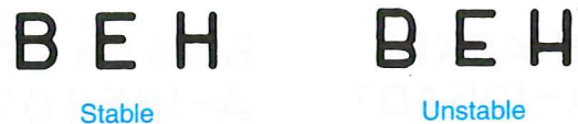
Figure 5-41. Some letters such as “B,” “E,” and “H” must actually be drawn with the horizontal bar just above the true center to make the letter appear correct. This makes lettering appear stable. If the bar is drawn at or below the true center of the letter, then the letter will appear unstable.
