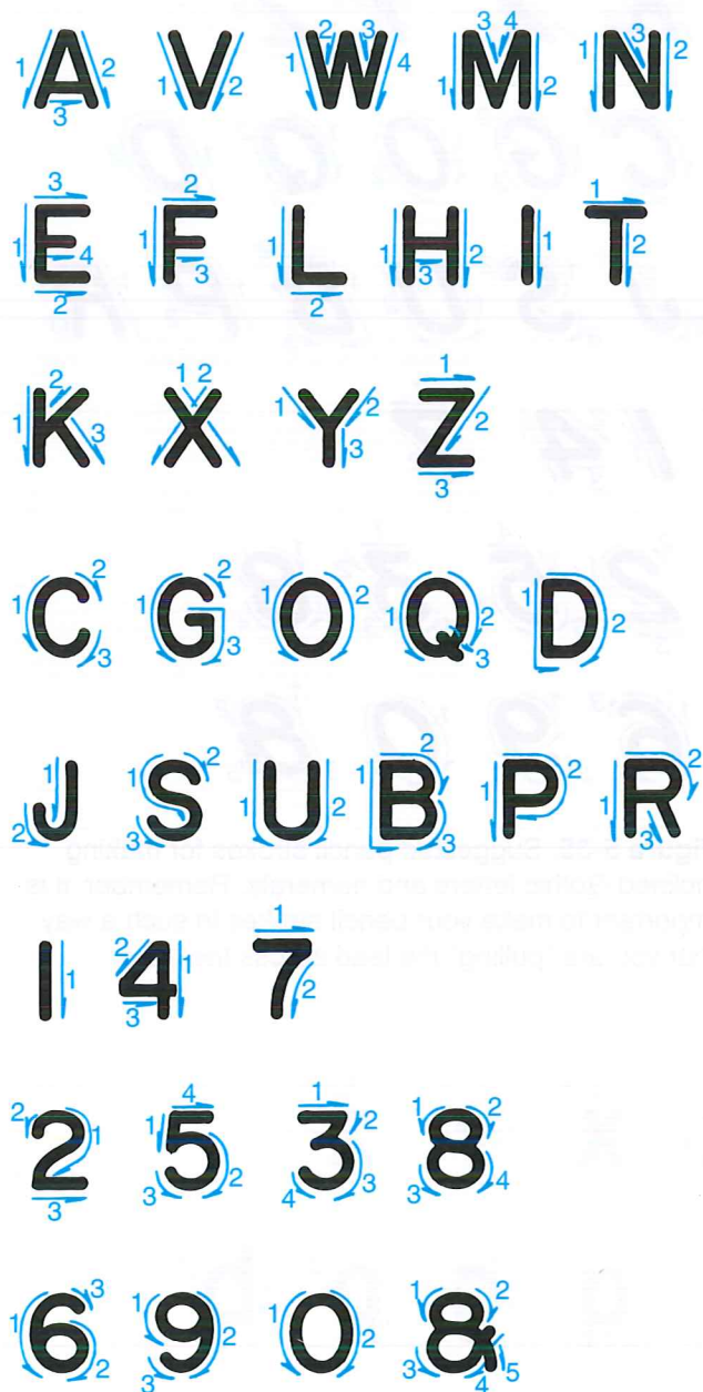
Figure 5-31. Suggested pencil strokes for making vertical uppercase letters and numerals. Remember, it is important to make pencil strokes in such a way that you are “pulling” the lead across the sheet, not “pushing” it.
