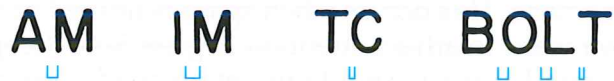
Figure 5-46. The total area between letters determines the spacing, not the total distance.
