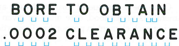
Figure 5-45. Equal spacing of letters results in poor composition and lettering that is hard to read.
