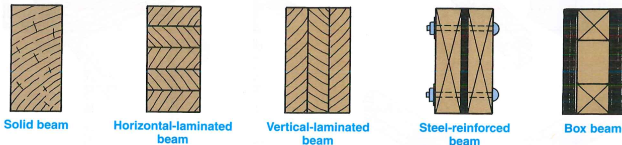
Figure 23-4. A variety of beams are used in wood post and beam construction.
