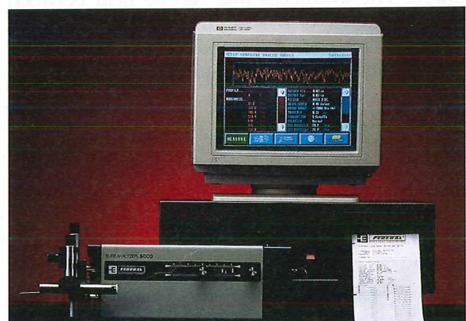
Figure 21-20. A surface roughness analyzer can measure up to 50 different surface finish parameters and display the results on screen. (Federal Products Co.)
