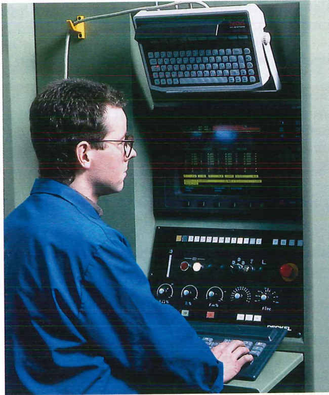
Figure 21-28. A machine operator uses a DNC computer keyboard to load the appropriate program for a part to be processed in a machining center. The computer on the machine is linked with the factory's central computer to make use of the information stored in a central database. (DLoG-Remex)
