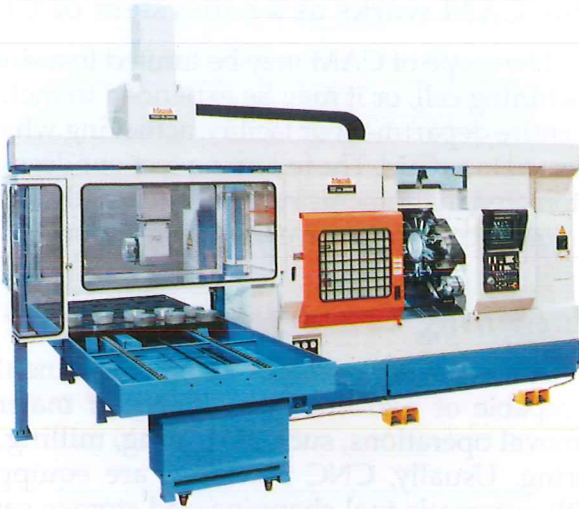
Figure 21-30. This dual-spindle turning center can work on both ends of a part simultaneously, as well as perform secondary operations such as drilling or tapping. Note the tool-changing turret next to the orange-colored safety cover (the cover has been opened to show the turret). Loading of parts to be processed is done automatically by the gantry-type robotic loader at the left end of the machine. (Mazak Corporation)
