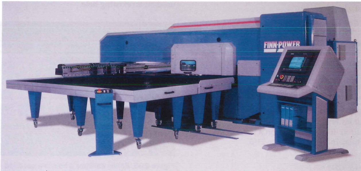
Figure 21-8. Large punch presses, like this 33-ton hydraulic precision turret model, are used to punch and form sheet metal. (Finn-Power International)
