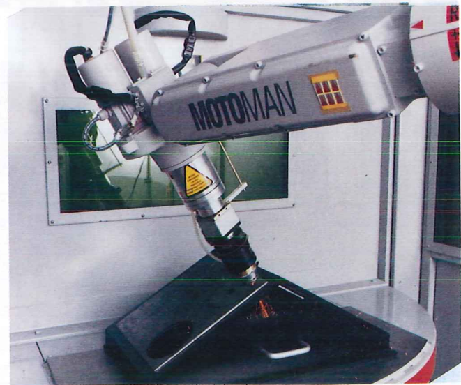
Figure 21-29. Robotics technology is widely used in industry today, especially for painting, cutting, welding, and assembly tasks. This robot arm is moving a laser cutting head, under CNC control, as it removes a precisely dimensioned circle of material from a metal plate. Fiber optic "light piping" channels the light beam from the laser generator to the cutting head. (Motoman)
