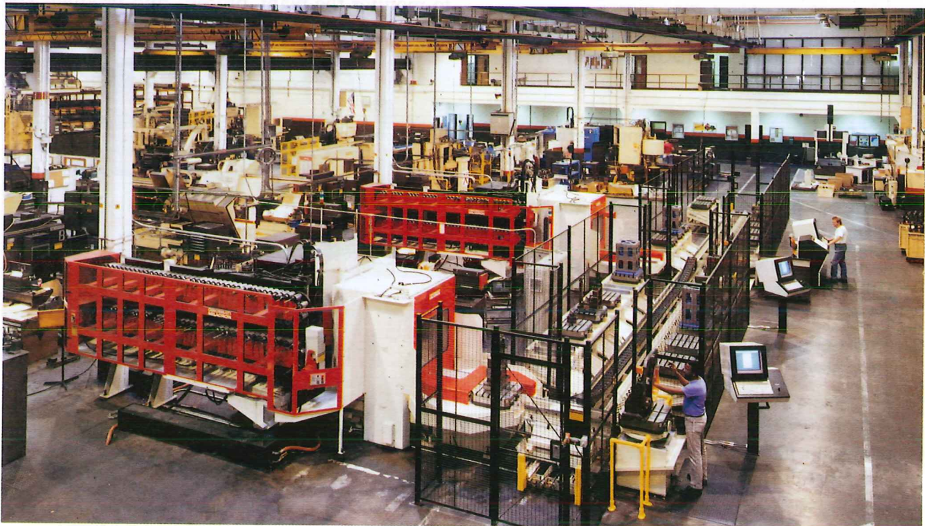
Figure 21-31. This flexible manufacturing cell consists of two horizontal machining centers served by a rail-guided pallet transporter. A load-unload station and a remote staging terminal are used with the 13 parts-holding pallets that help ensure continuous flow of material through the machining centers. (Cincinnati Milacron)
