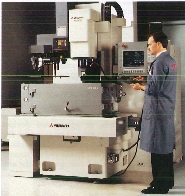
Figure 21-26. A CNC electrical discharge machine. The operator is using a multifunction remote control for the unit. (Mitsubishi)
