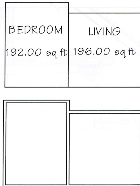
Figure 3-20. Some AEC CAD programs can take a space diagram (top) and create a floor plan from it (bottom).
