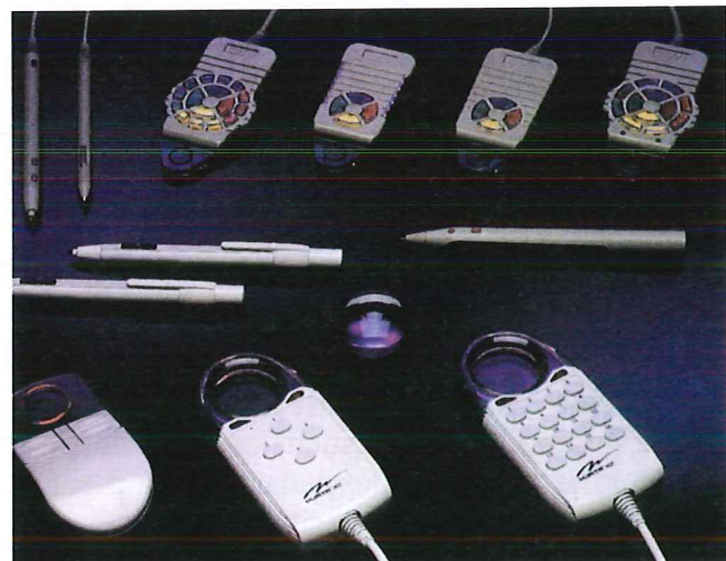
Figure 3-9. Digitizer pucks are available in a variety of configurations. The light pens shown here are another type of input device. (Kurta)
