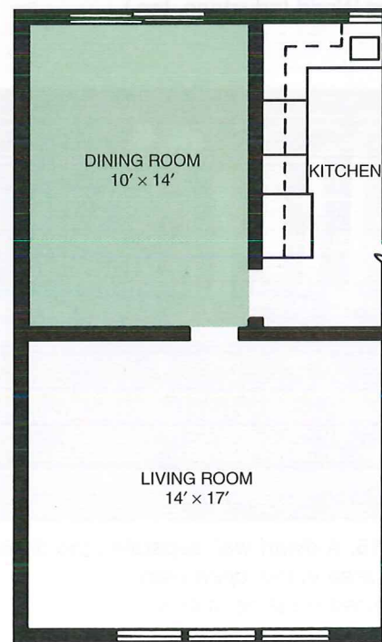
Figure 8-16. A wall separates the living and dining rooms. This is a closed plan because there is little chance for overflow between the two rooms.
