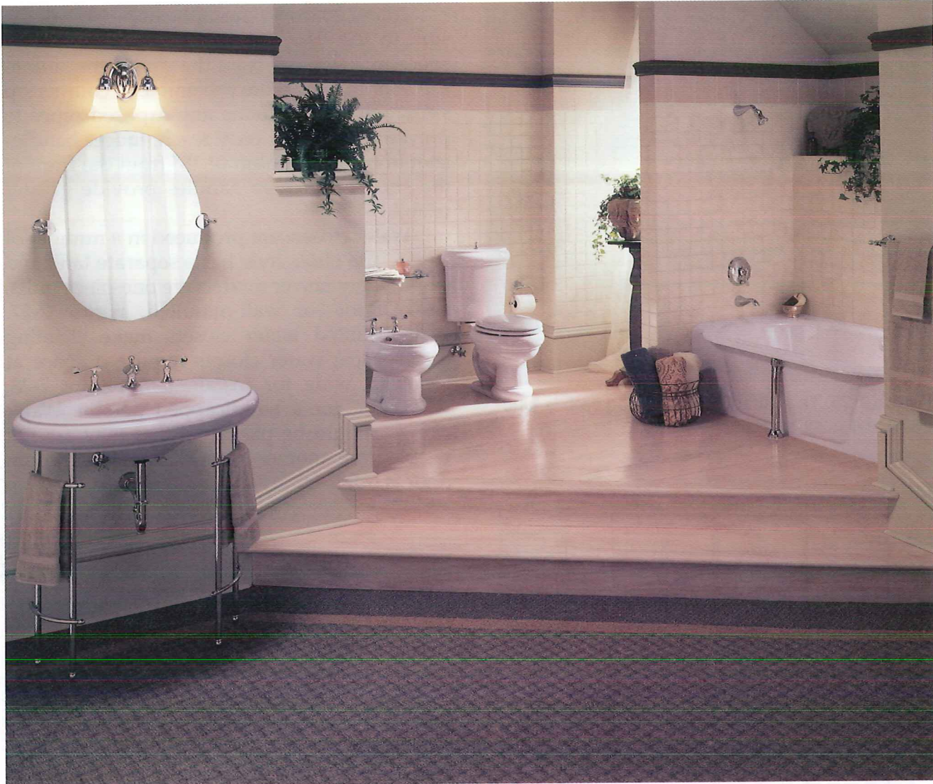
Figure 7-23. A lavatory should have a mirror above it. Avoid placing a lavatory or water closet under a window. (Photo courtesy of Kohler Co.)
