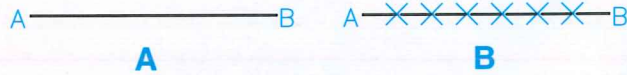
Figure 6-10. Using the Divide command to divide a line into an equal number of segments.
