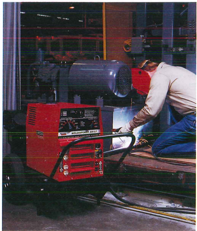
Figure 26-2. In arc welding, heat is generated by an electric arc between a metal electrode and the parent metal. In some arc welding processes, metal is added to the parent materials being joined. (Lincoln Electric)
